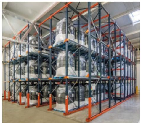
FUNCIONAM COM SISTEMA LIFO (*LAST IN, FIRST OUT*) OU FIFO POR LOTES QUANDO SE TEM MAIS DE TRÊS RUAS POR REFERÊNCIA.
